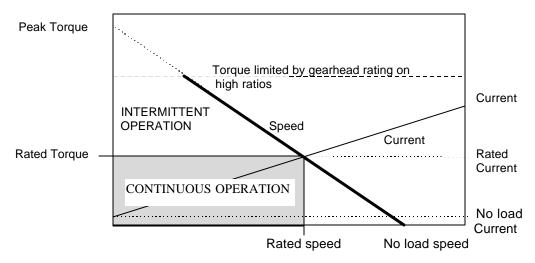
As will be seen from above, the relationship between current and torque is constant throughout the entire speed range thereby enabling accurate control to be obtained. Furthermore, the low internal losses of both the motor's commutation system and the precision gear train results in low no-load operating current and high overall efficiency.
