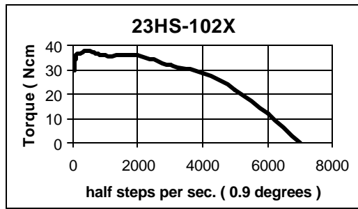
Coils in parallel, 1.2 amps per phase
