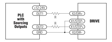
Connecting to PLC with Sourcing (PNP) Outputs
