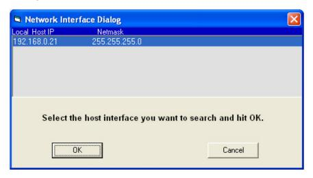
Normally, Drive Discovery will only detect one network interface card (NIC), and will select it automatically. If you are using a laptop and have both wireless and wired network connections, a second NIC may appear. Please select the NIC that you use to connect to the network to which you've connected your drive. Then click OK. Drive Discovery will notify you as soon as it has detected a drive.
