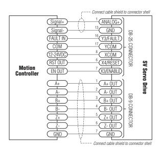
Connecting a Motion Controller with Analog (±10V) Output
