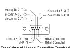
Front View of Motion Controller Feedback (MCF) connector
