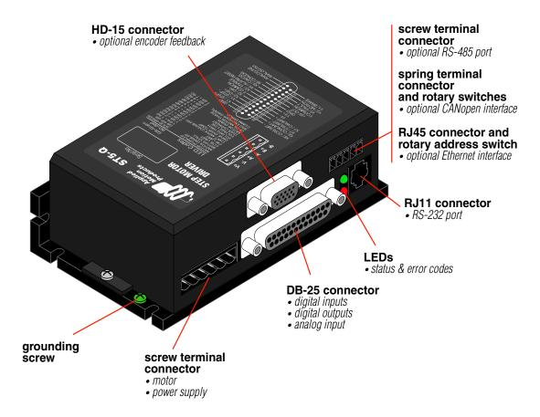
Drive ground and PC ground can be at different potentials, be sure these two grounds are at the same potential or the ground pin of the serial port can become damaged, requiring repair.
