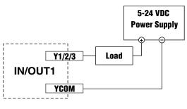
Sinking Output Using Y1, Y2, Y3
