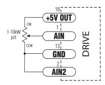
**Connecting a Potentiometer to Analog Input 1**
