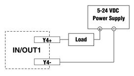
Sinking Output Using Y4
