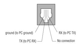
Pin Assignments of the PC/MMI Port (RJ11 connector)
