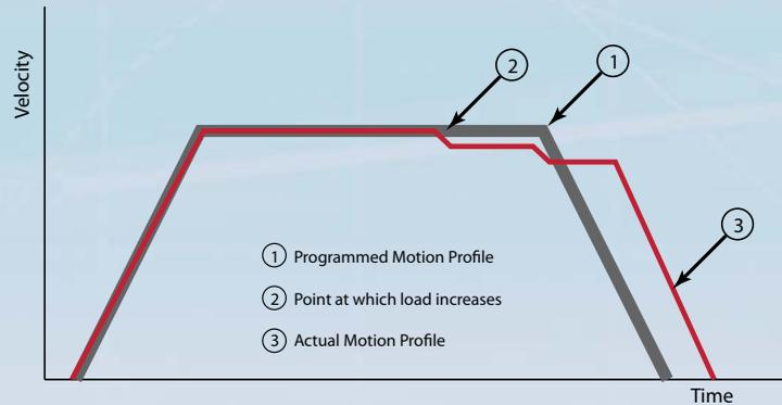
Figure 2: Diagram showing the Stall Prevention process
