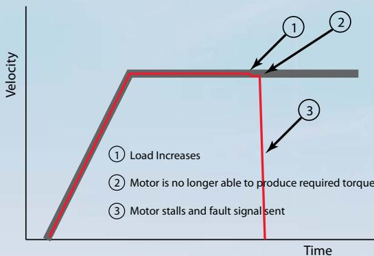
Figure 1: Diagram showing the Stall Detection process
