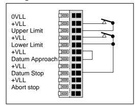
In applications where space is limited the end of travel limit switches may also be used as the datum stop switch. In the example shown the lower limit switch is also connected to the datum stop input and the controller is configured to utilise the high speed datum approach facility.
