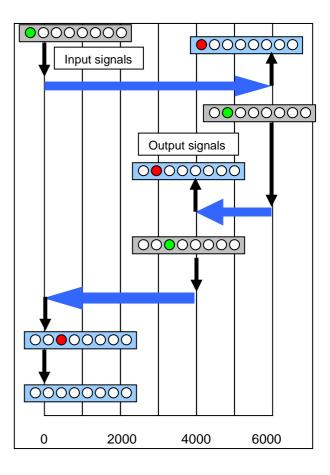
By sending command: 1xs1 (execute sequence one) the above motion programme is executed once. By adding a 1xs1 command at the end of a sequence before the 1es command, the sequence can be made to continuously repeat.
