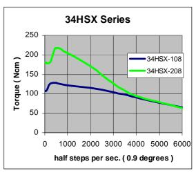
Ensure the drive current is set appropriately for the rating of the motor. Standard configuration is set at 3.5 Amps.
