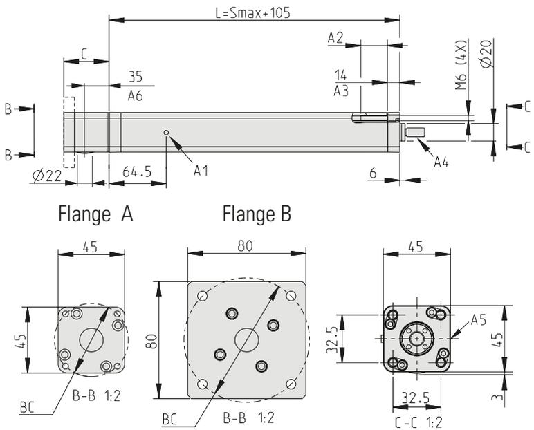
A1: grease port A2: M6 thread, max. depth 30 mm A3: no thread
