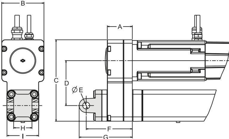
The rear clevis consists of a bracket and comes mounted from the factory if the ordering code states that the unit shall be equipped with one. It can also be ordered as a separate part using the part number in which case it is delivered with the necessary screws to attach it to the actuator.
