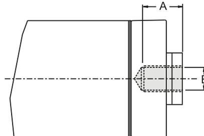
The female threaded rod end comes mounted from the factory if the ordering code states that the unit shall be equipped with one.
