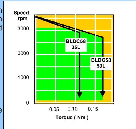
Speed regulation from 100-3000 rpm is obtained using the MSA933 motor speed control module.
