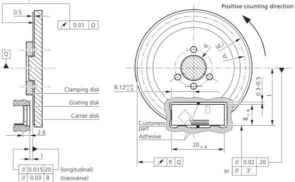
Bonding of the EPIFLEX measuring module outside the 3 contact pads on both longitudinal sides.
