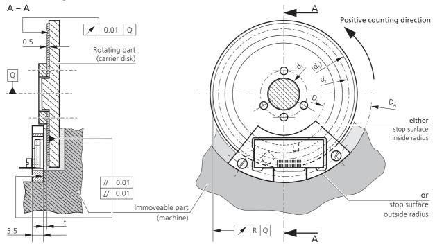
Dimensions and tolerance limits to be observed by the user to ensure proper functioning, without angular error being taken into account
