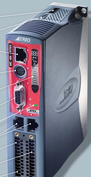
The MC4N-RTEX is dedicated to running remote servo drives via Panasonic's RTEX Real Time EXpress automation bus. It is based on an up-rated version of the 532MHz ARM 11 processor which makes it ideal for high axis count machines or robotic applications.
