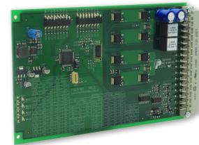
type inputs. Four surface mounted status LEDs indicate power, drive disabled, over-temperature and overload faults.
