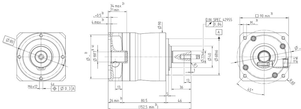
Up to 28<sup>4)</sup> (H) clamping hub diameter
