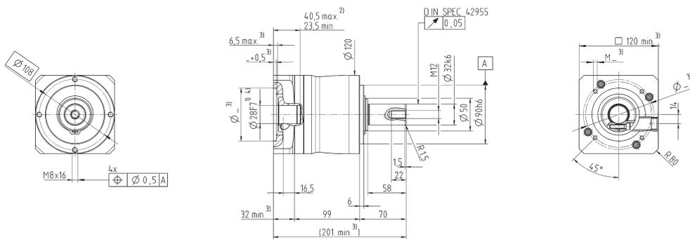
Up to 38<sup>4)</sup> (K) clamping hub diameter
