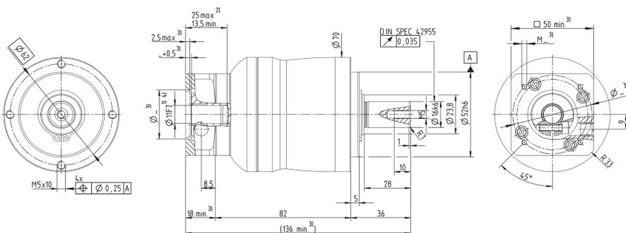
Up to 14<sup>4)</sup> (C) clamping hub diameter
