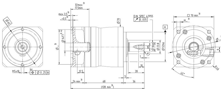
Up to 19<sup>4)</sup> (E) clamping hub diameter
