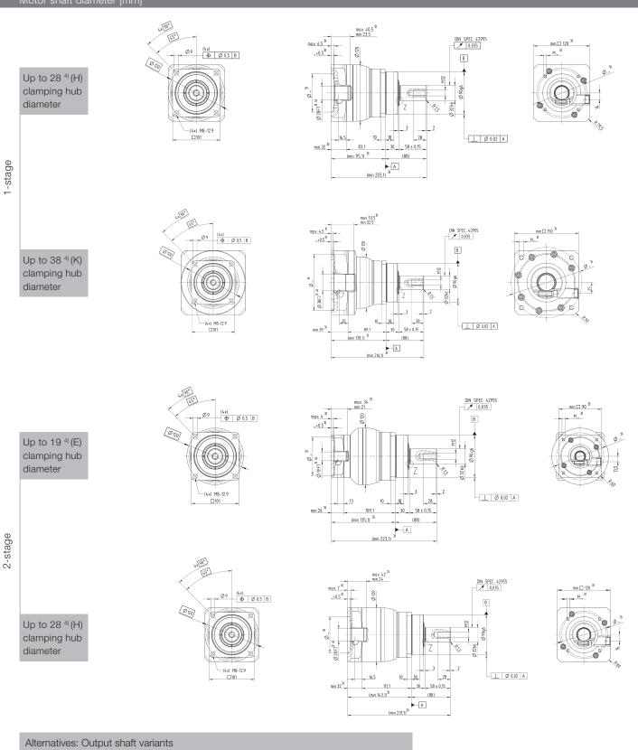
Output shaft with key E = key as per DIN 6885, sheet 1, form A
