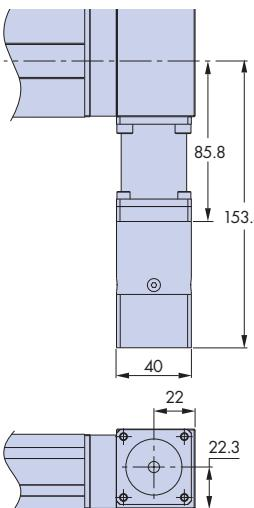
Hepco will supply fitted gearboxes with ratios from 3:1 to 512:1 complete with input flange to suit your motor.
