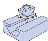
T-slot cover (supplied fitted in each of the T-slots) = 1-242-1037
