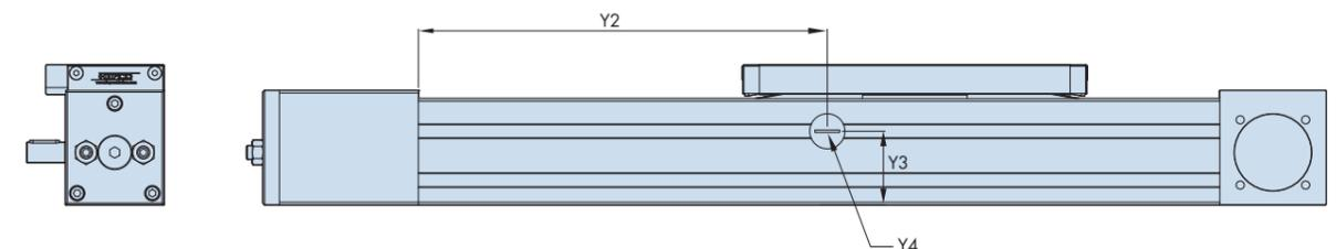
Re-lubrication of the ball guide carriage block is via an access point in the side of the beam (see above), which is closed off with a threaded plug. The lubrication interval depends on the length of stroke, speed and duty. For further details regarding lubrication procedures please contact Hepco's technical department.
