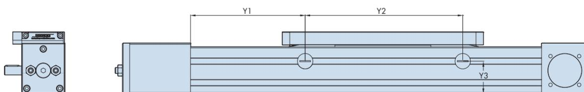
Re-lubrication of the ball guide carriage blocks is via two access points in the side of the beam (see above), and closed off with a threaded plug. The lubrication interval depends on length of stroke, speed and duty. For further details regarding lubrication procedures please contact Hepco's technical department.
