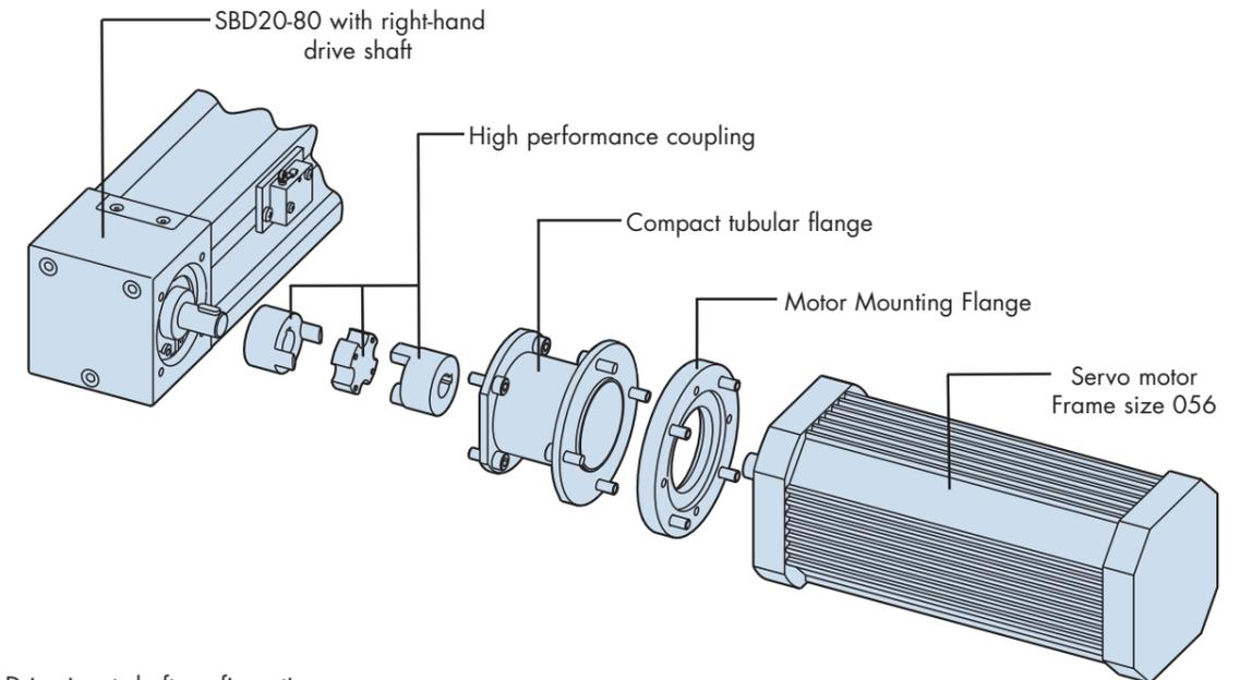
Drive input shaft configurations
