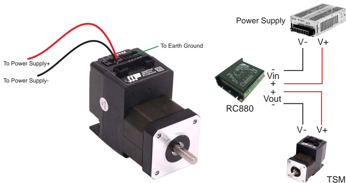
Applied Motion Products offers two matched power supplies for use with the TSM. A 24VDC, 150W(P/N PS150A24) and a 48VDC 320W(P/N PS320A48). These power supplies have current over load capability making them ideal for use. (To use with a switch power supplier, a RC880 regen must be connected in system)
