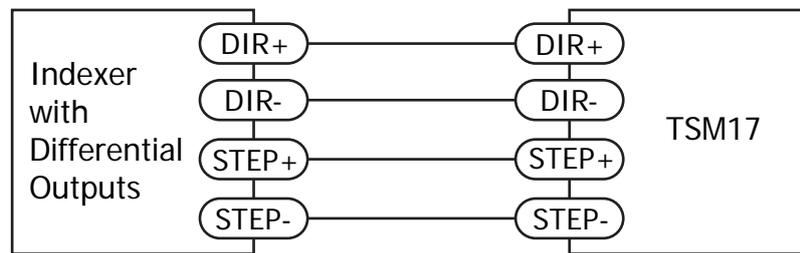
Connecting to Indexer with Differential Outputs
