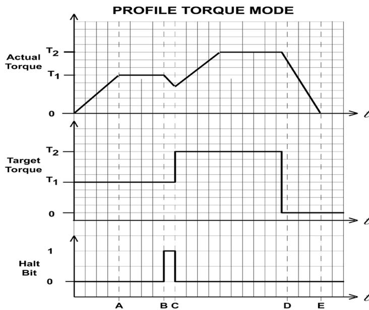
Figure 18: Profile Torque Mode
