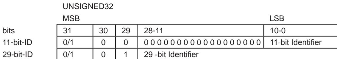
Figure 7: Structure of the EMCY Identifier entry
