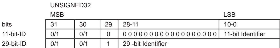
Figure 9: Structure of PDO COB-ID entry
