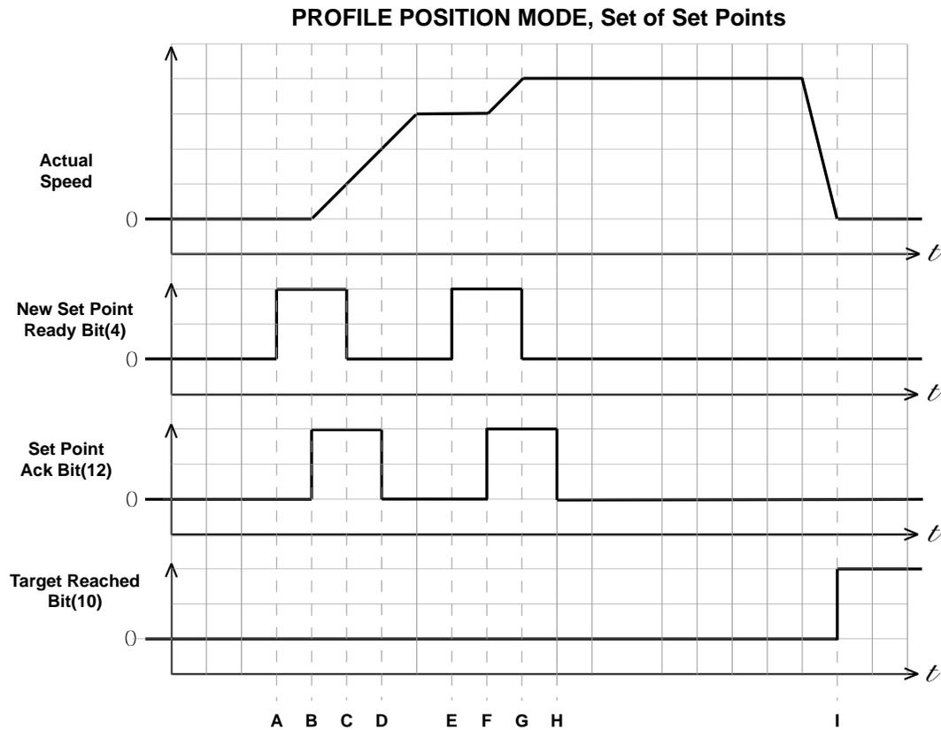
**Figure 15: Multiple Set-Points, Immediate Change in Motion**
