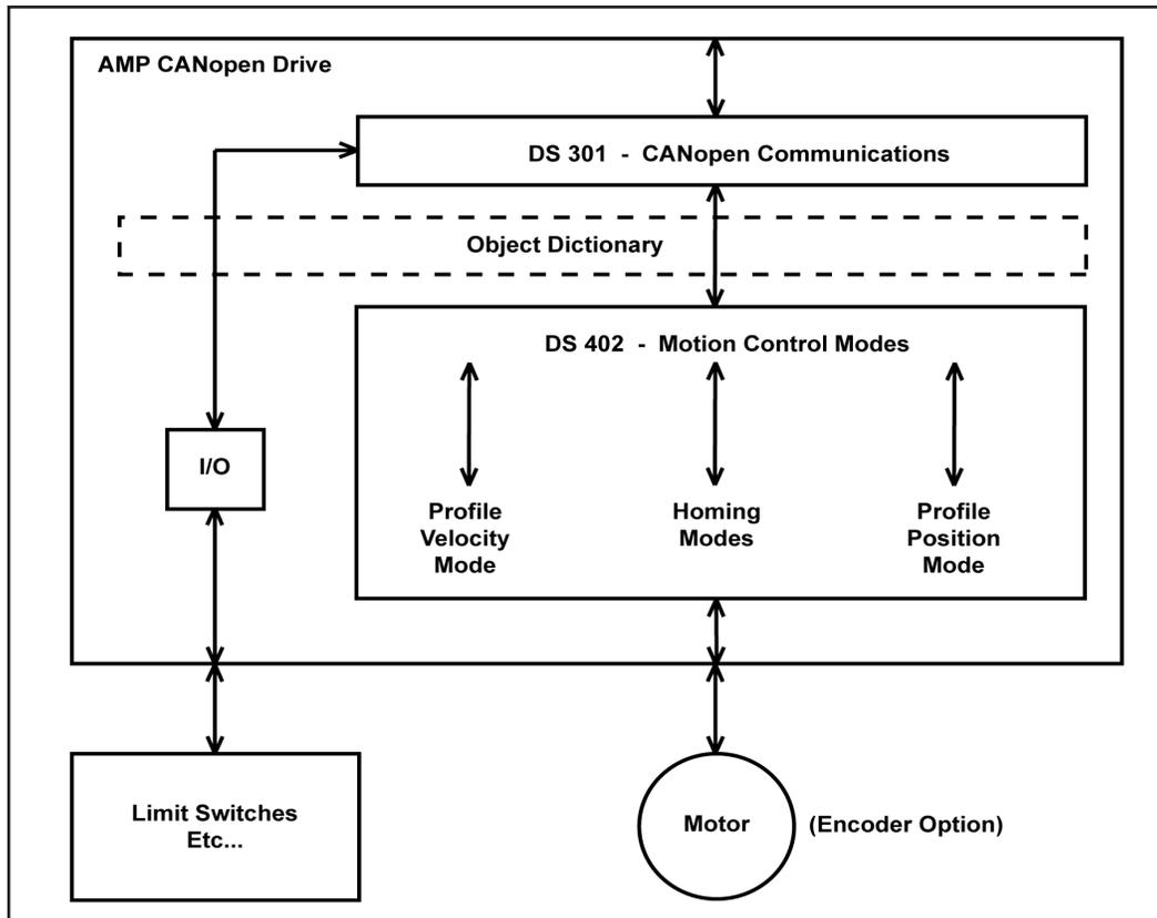
Figure 4: CANopen Drive - Motion Control Modes
