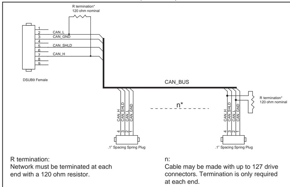
Figure 3: Wiring Schematic
