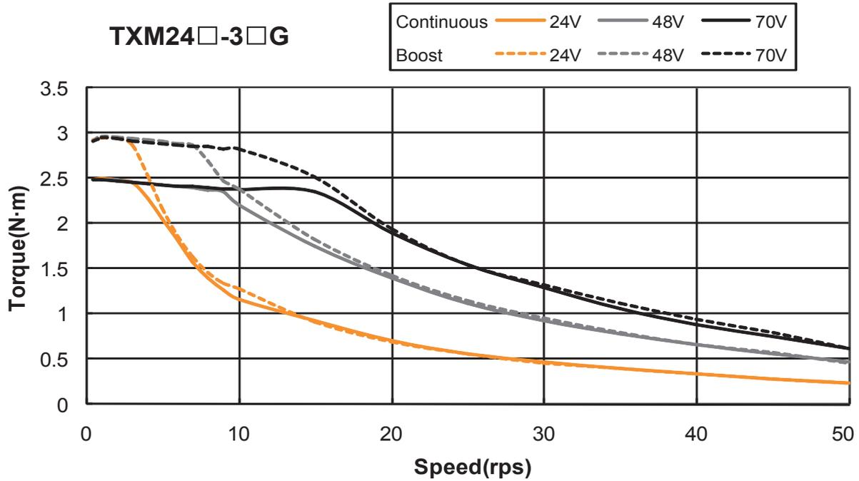
Note: all torque curves were measured at 20,000 steps/rev.
