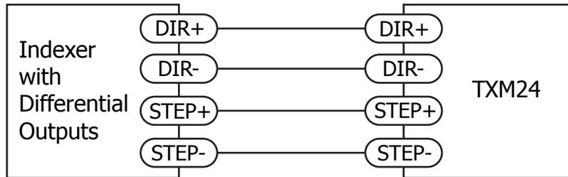
Connecting to Indexer with Differential Outputs
