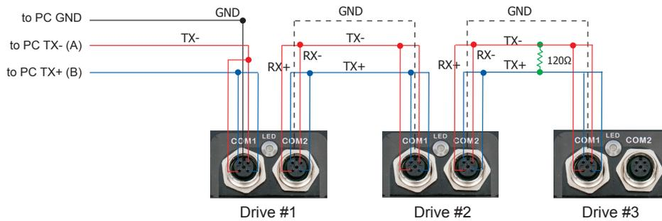
**NOTE: If the PC does not have an RS-485 serial port, a converter is required. You can contact Applied Motion Products to buy a USB to RS-485 converter.**
