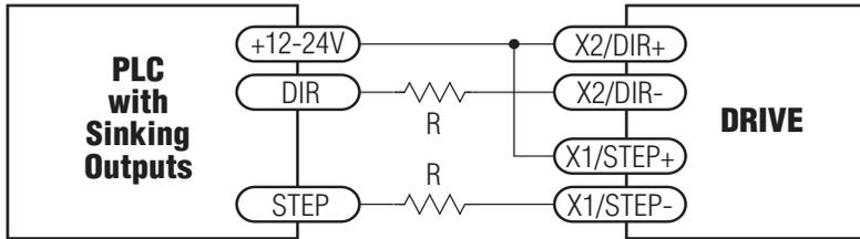
**Connecting to PLC with Sinking (NPN) Outputs**
