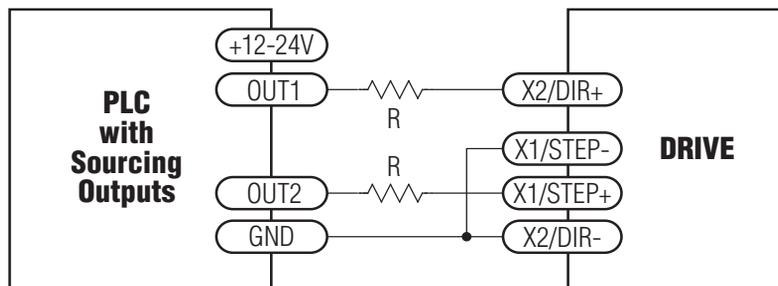
**Connecting to PLC with Sourcing (PNP) Outputs**
