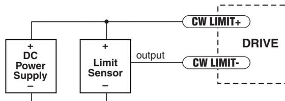
If the sensor output goes low at the limit, select the option “closed” (in the software). If the output is open, or high voltage, choose “open”.
