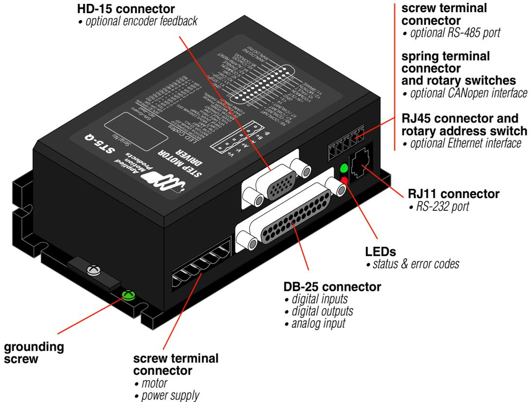
**Drive ground and PC ground can be at different potentials, be sure these two grounds are at the same potential or the ground pin of the serial port can become damaged, requiring repair.**
