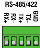
It's not recommended that both the RS232 and RS485 ports be active (connected) at the same time. Only one serial port should be physically connected at any time.
