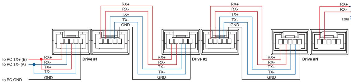
**NOTE: If the PC does not have an RS-485 serial port, a converter is required. You can contact Applied Motion Products to buy a USB to RS-485 converter.**
