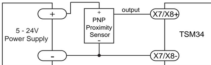
Connecting a PNP type Proximity Sensor to an Input
