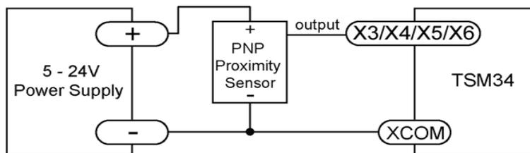
Connecting a PNP type Proximity Sensor to an Input
