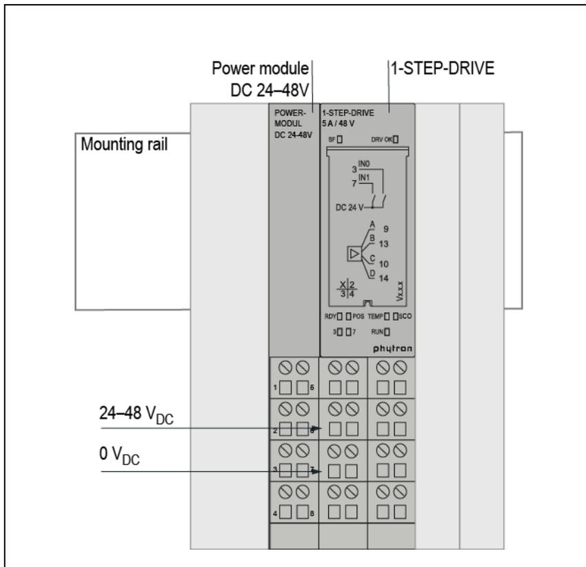
Fig. 6: Connection of the DC24-48V power module
