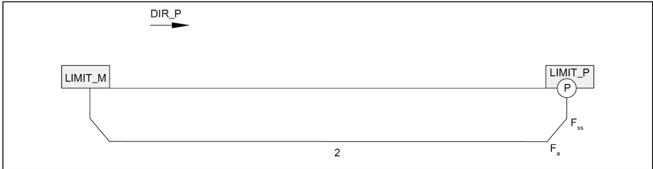
Fig. 28: Start at the limit switch LIMIT\_P
