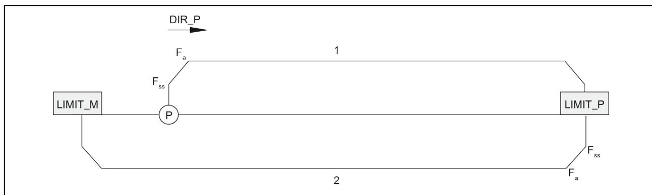
Fig. 27: Start within the allowed traverse range
