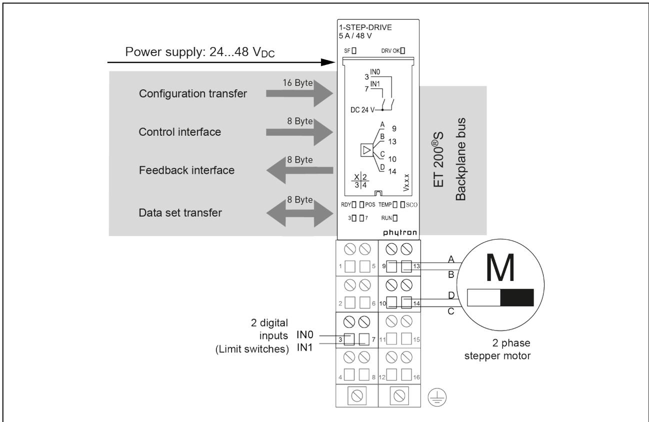
Fig. 11: Terminal assignment
