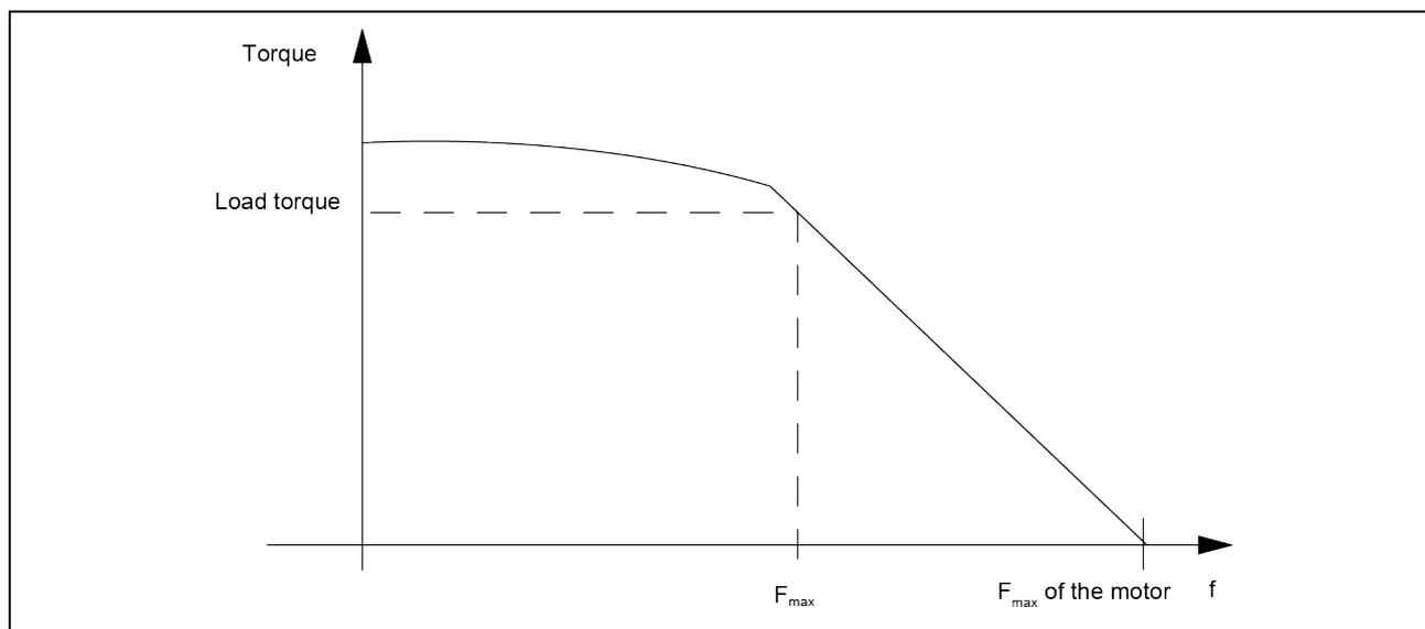
Fig. 22: Torque Characteristic Curve of a Stepping Motor
