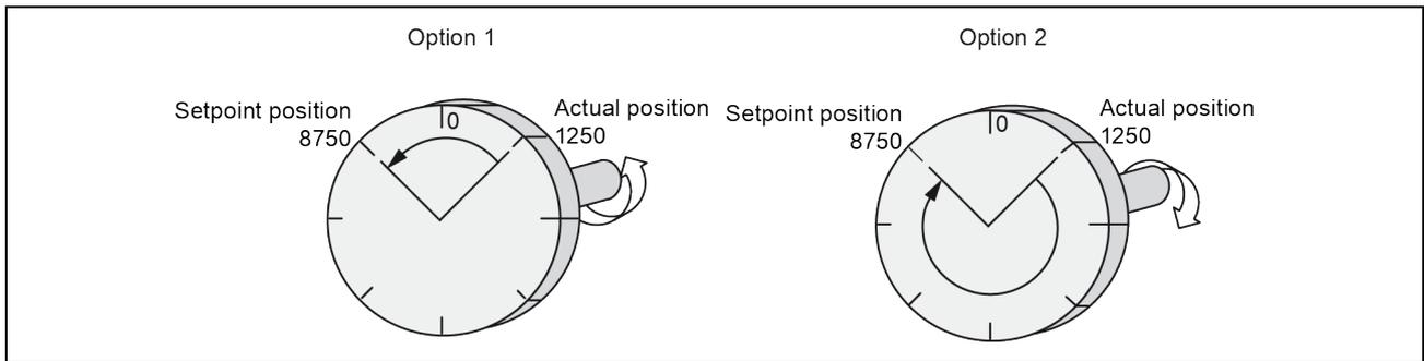
Fig. 32: Absolute incremental mode with modulo axis
