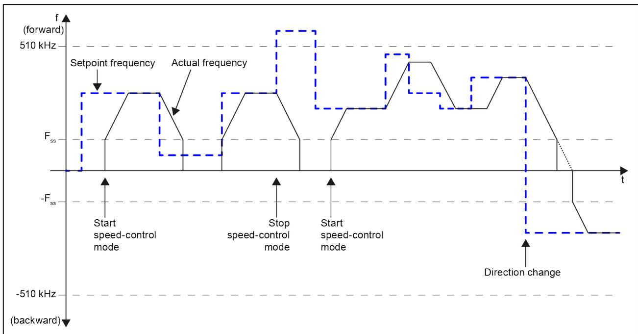
Fig. 29: Velocity control mode with modulo axis
