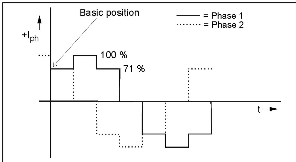
Fig. 39: Motor phases in basic position (half step)
