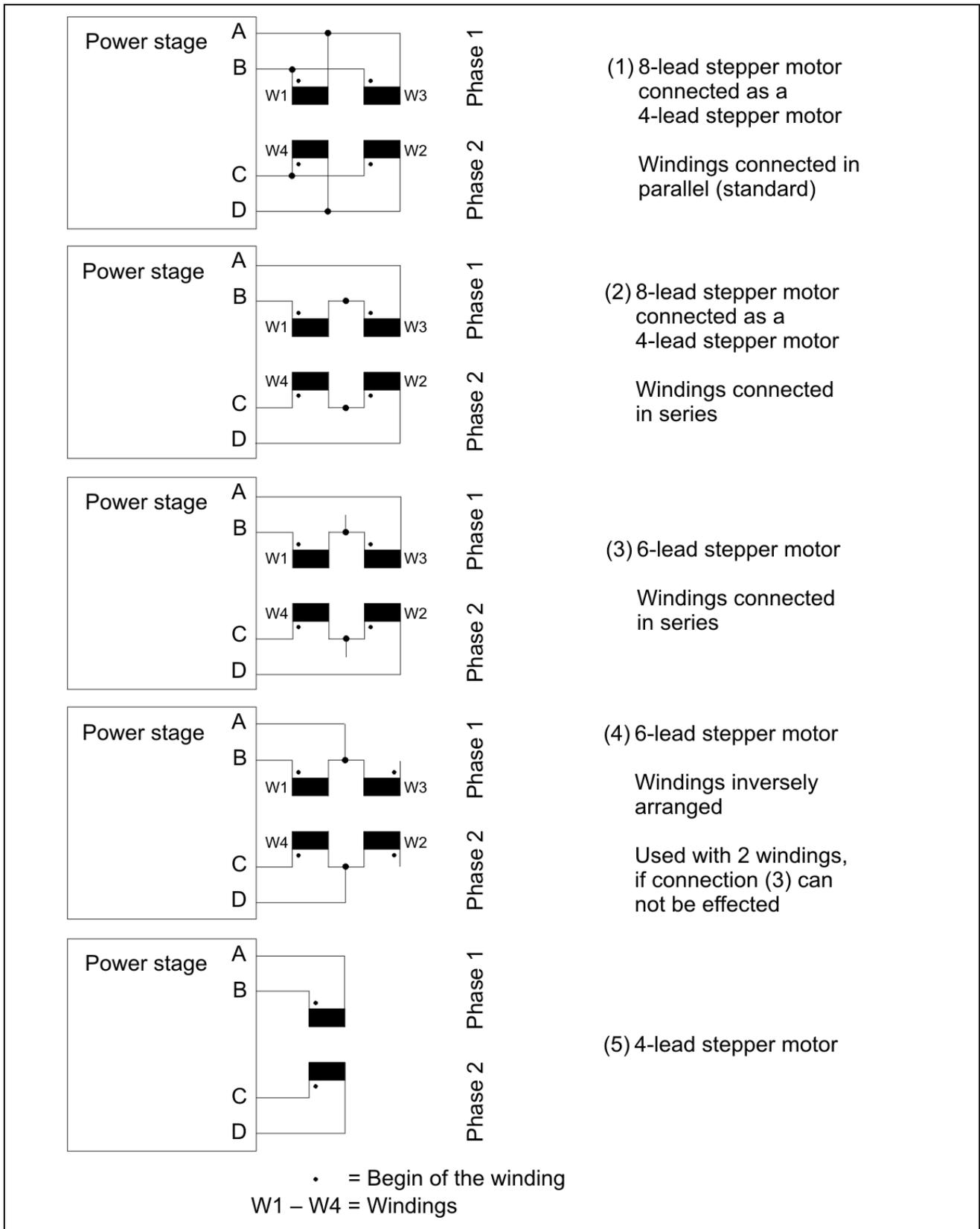
Fig. 12: Connection diagrams for 4-, (6-) and 8- wire stepper motors
