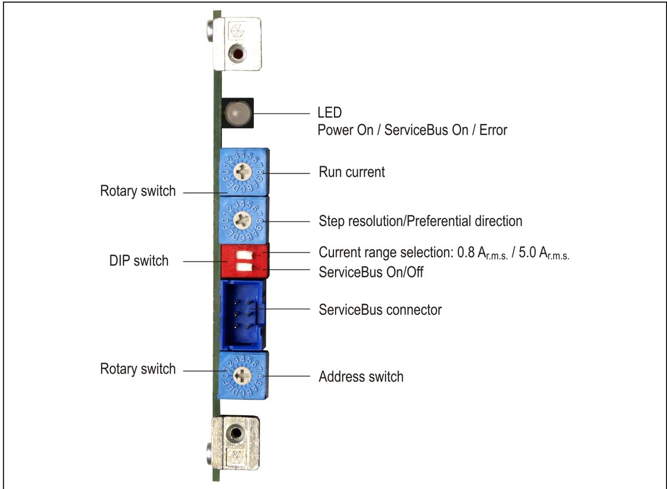
Fig. 1: Control components
