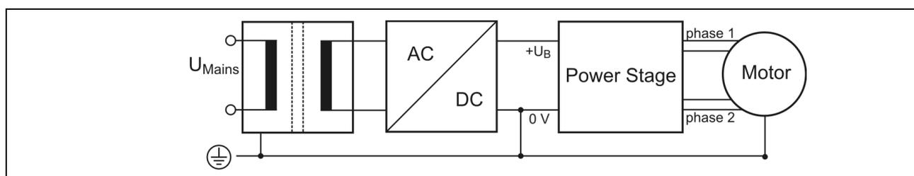
Fig. 4: PELV – Grounding: 0 V and Motor
