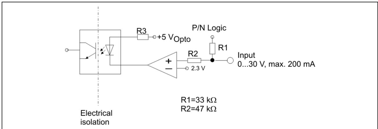
Fig. 20: Input circuit "electrical isolation"
