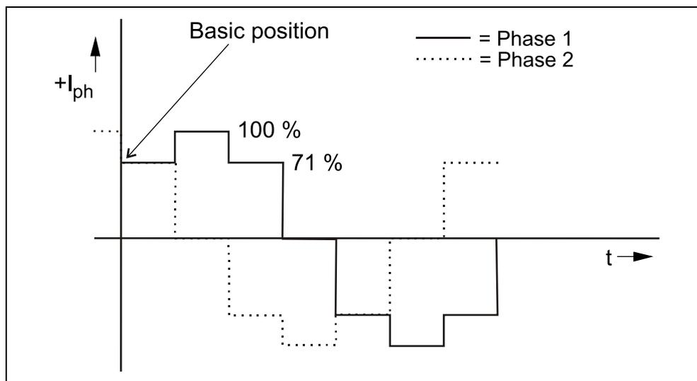
Fig. 22: Motor phases in basic position (half step)
