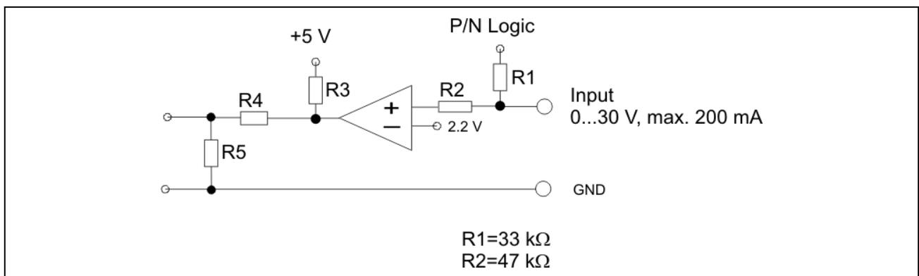
Fig. 21: Input circuit "without electrical isolation"
