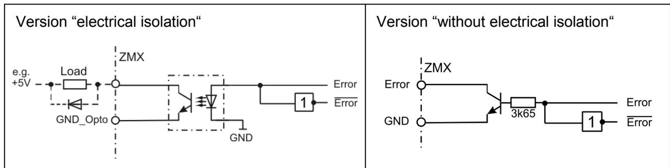
Abb. 1: Output wiring diagram
