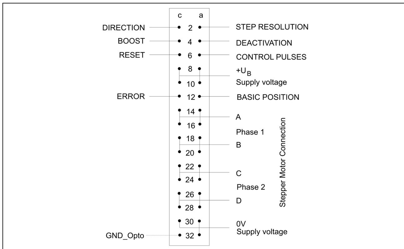
Fig. 13: 32 pin VG connector, type D acc. to DIN 41612
