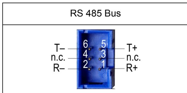
Fig. 12: ServiceBus connector type Tyco Electronics 2-1761605-1/609-0607
