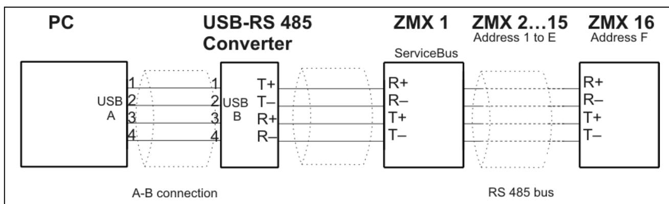
Fig. 18: Connection PC -> ZMX<sup>+</sup> via USB/RS 485 converter
