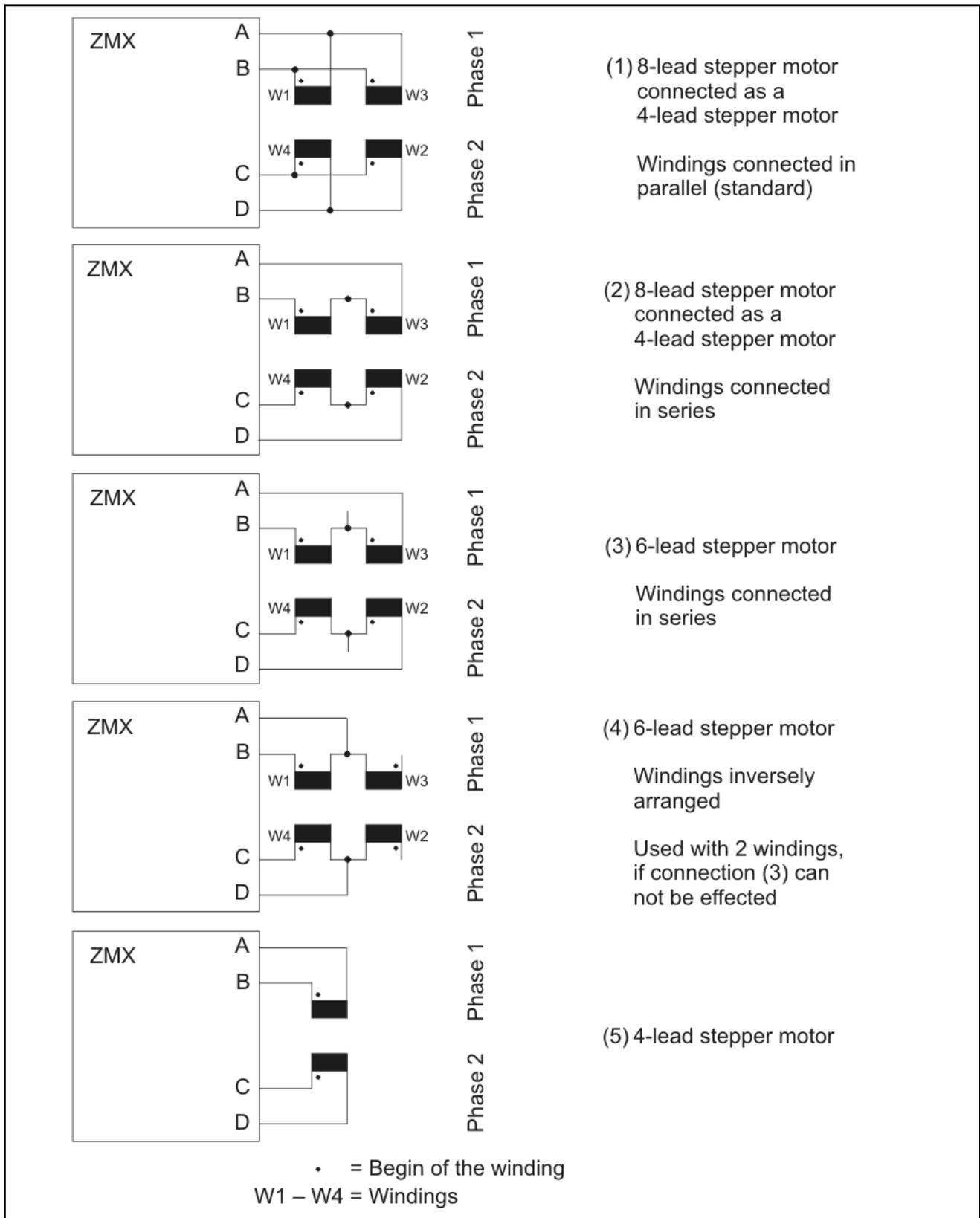
Fig. 11: Connection diagrams for 4-, 6- and 8- wire stepper motors
