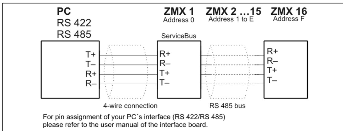
Fig. 19: Connection PC -> ZMX<sup>+</sup> with RS 422/RS 485 interface
