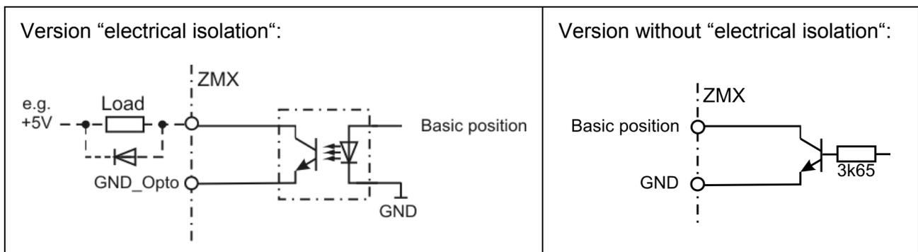
Fig. 23: Output wiring "BASIC POSITION" without electrical isolation
