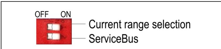
Fig. 16: DIP switches at the front side
