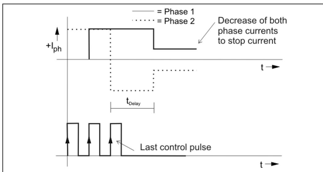
Fig. 25: Decrease to stop current after the last control pulse (full step)
