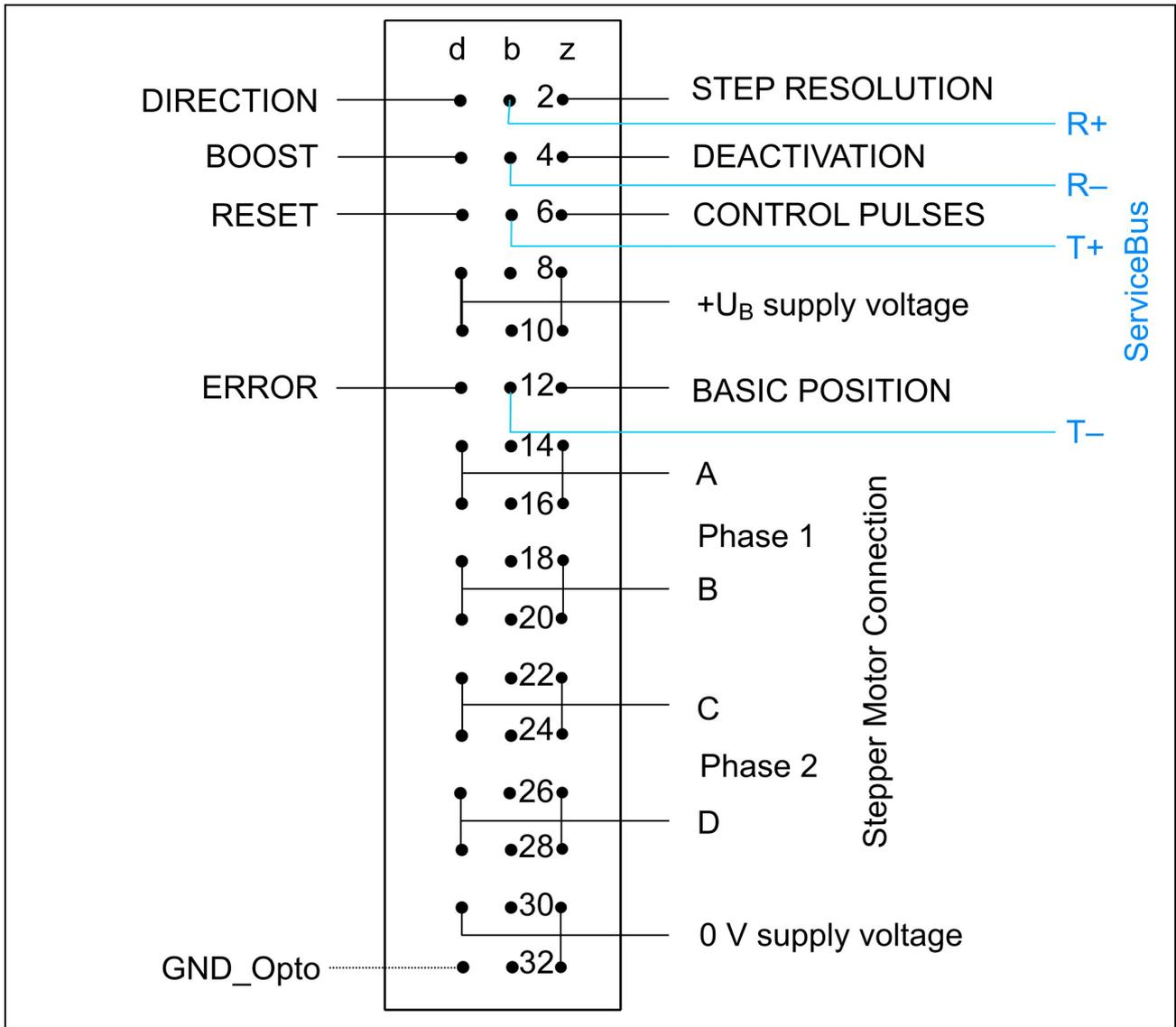
Fig. 14: 48 pin VG connector, type F acc.to DIN 41612
