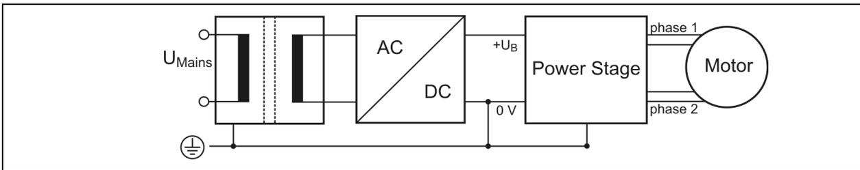
Fig. 5: PELV – Grounding: 0 V and Power Stage
