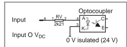
The 6 digital outputs are optically isolated and the rated output current is 50 mA.
