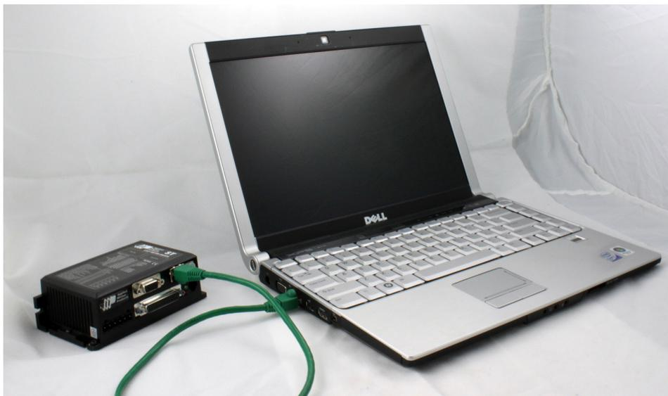
You don't need a special "crossover cable"; the drive will automatically detect the direct connection and make the necessary physical layer changes.
