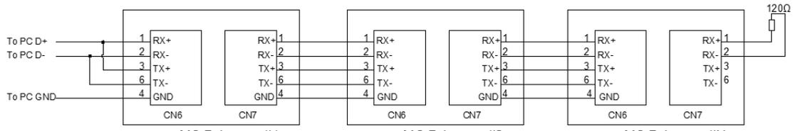
NOTE: For the 120 ohm terminating resistor, we recommend crimping the resistor leads into an RJ45 8 pin modular plug.
