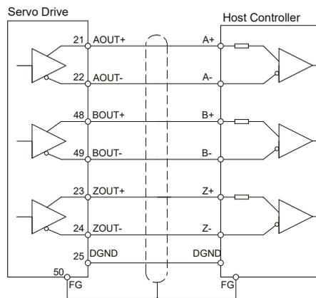
NOTE: Please make sure the host controller and the servo drive are connected to a common ground.
