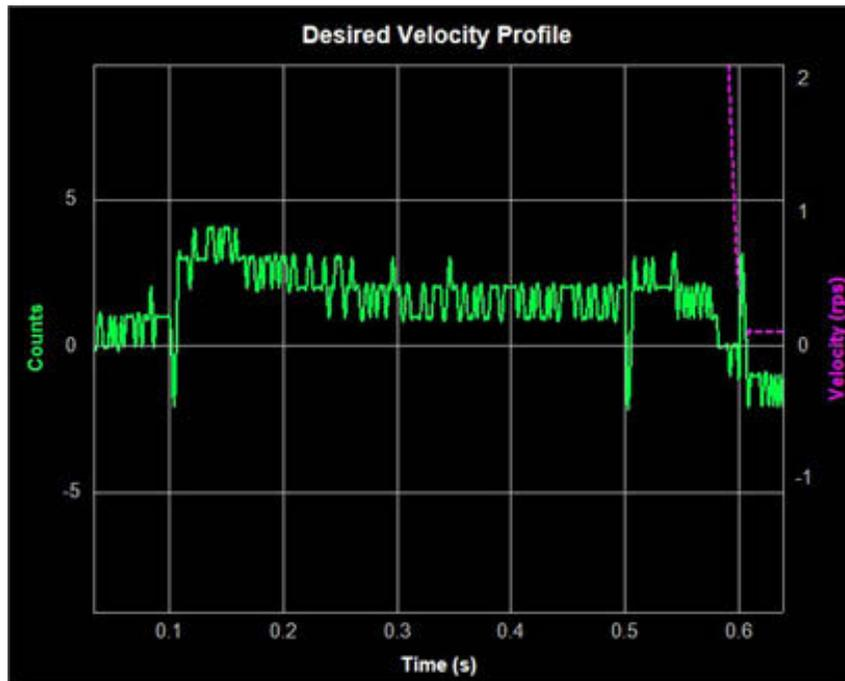
As shown below, if the KF value is set appropriately, the position error during acceleration and deceleration will settle very quickly, and position error of  $\pm 1$  count can be achieved during constant velocity as well as when the motor comes to rest at its target position.
