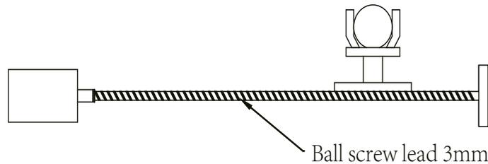
Distance for screw lead move requirement = 4mm.
