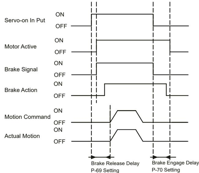
The Brake Output (BO) setting can be configured with the SVX Servo Suite software or with parameter P-67(BO), as shown in the table below. Brake disengage delay and engage delay times can be configured via SVX ServoSUITE®, or by changing parameters P-69 (BD) and P-70 (BE) directly from the drive.
