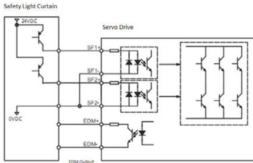
Note: the EDM output, must be limited to 24VDC(max), 100mA(max), limit current as necessary.
