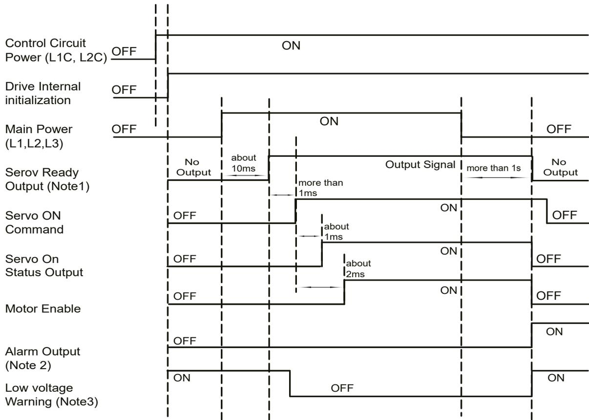
Note 1: When the Main power circuit is powered off, it will take more than 1 second for the internal capacitor to discharge before Servo Ready signal is OFF
