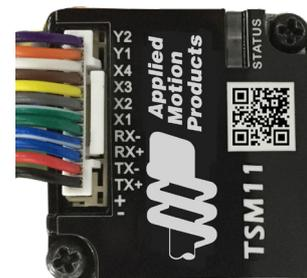
**Note: All digital inputs & outputs are referenced to the power ground pin 12 – (V-).**
